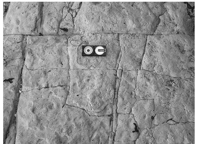
Fig. 9. Top view of a layer at the Pillar outcrop, the systematic joint set is the N10° joint set, parallel to the long side of the compass. Most, but not all, of the N120° joints abut on the first joint set.
